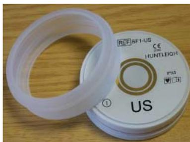
The transducers are protected against damage by a silicone bumper. Never operate the transducer without this protective bumper. It can be removed for cleaning if required. Refer to Section 6.2 for instructions.
