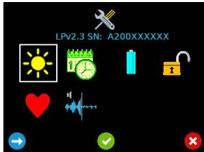
When a Vascular probe is attached, the Setup screen gives access to the Heartrate Display Selection Screen and DDNR Hiss Suppression Screen.
