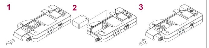
Note: Remove the battery if the unit is not likely to be used for some time.
