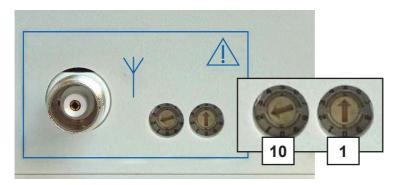
Use the code-switches on the rear panel of the receiver to select the new channel number.
