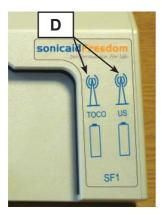
The transmission indicators are located on the upper right corner of the receiver (D). These indicators show the status of TOCO and US transducer transmission:
