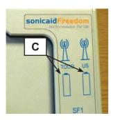
Once a transducer has been identified by the receiver, the corresponding battery indicator (C), shows the battery level during operation and the recharge level during charging. Each LED represents about a quarter of the capacity. When the battery is fully charged, all 4 LEDs are continuously on. An operating time of about 16 hours is available on a full charge. A complete charging process takes approximately 2.5 hours.
