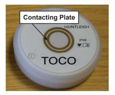
On the top surface of the transducer is a contact plate. The two connecting rings connect to the charging pins on the receiver when the transducer is docked for charging. All rings are internally disconnected during operation.
