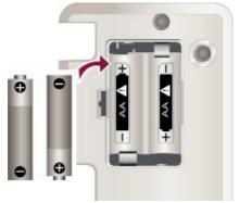
Insert the batteries according to the diagram, observing polarity.
