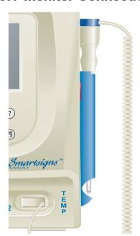
Connect the temperature probe to the front panel socket marked TEMP and place the sensor into its holder on the side of the unit.
