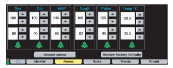
Use the ▲▼ keys to adjust the limits as necessary.
